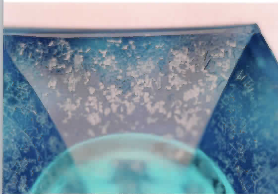
(Above): Macro-photograph of the underside of the hexagonal stopper of bottle featured in picture 5. The stopper consists of six concave panels, rising upward in an almost trapezoidal form. Captured are two common characteristics of crizzling, namely, tiny formative crystalline structures in the central panel; and crack-like lines in the two flanking panels. Frank and Elizabeth Creech, bottle owners and photographers.
